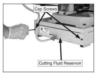
Figure 14. Opening cutting fluid reservoir.
